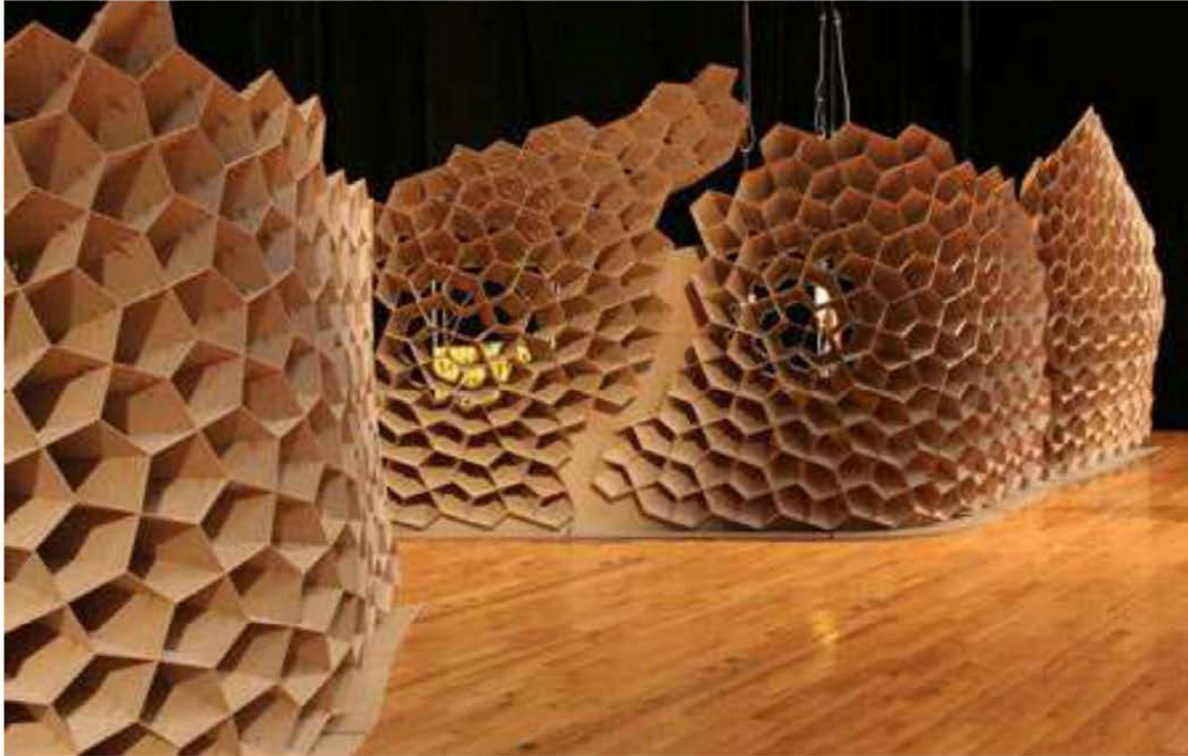
Exhibition stand with an irregular honeycomb MDF structure Institute for Lightweight Structures and Conceptual Design (ILEK) at the University of Stuttgart
